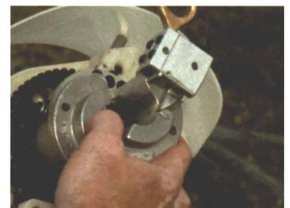
STEP # 4. Choose the bushing with the number that matches the cable gage number that indicated the cable size in the previous step. Insert the bushing into the tool head by pushing the retaining spring in and sliding the bushing into the bushing holder. The bushings will only go in one way because they have different diameter holes that fit on different size pins. Slide the bushing half without the blade into the tool first. Then repeat the operation for the bushing half with the blade.
