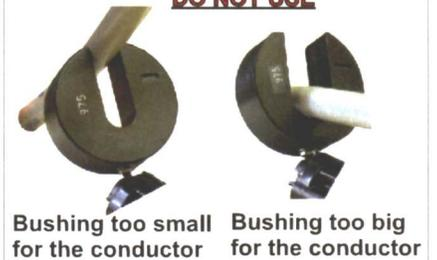
STEP # 3. Determine the bushing needed by using the cable gage and a grip all stick (shotgun). Push the gage on the cable. The cable should go half way down the gage as shown above. If the cable will not go into the gage, the bushing is undersized and should not be used. If the cable drops fully into the gage, the bushing is oversized and should not be used.
