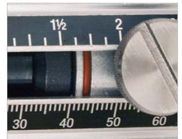
Thumb screw & strip gauge to adjust to precise stripping lengths.
