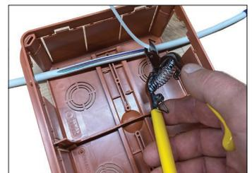
Safely access inner fibers in seconds.
