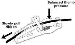
Apply gentle thumb pressure to add drag. Pull ribbon along arc towards blade edige to slice matrix. Slice 1 matrix node every 5 seconds or slower. WARNING: This tool should not be used on live electrical circuits. It is not protect against electrical shock.
