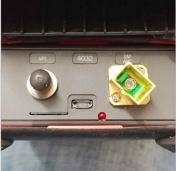
The factory-configured top panel features a VFL port, a laser port with multiple adapter options, and space for future expansion ports.
