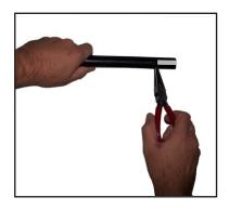
3. Peel scored segments with needle nose pliers or other suitable tool.
