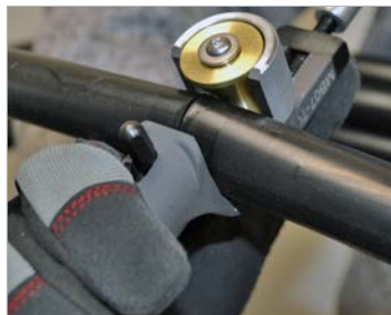
Ergonomic tool handle provides additional leverage during ring cutting operations.
