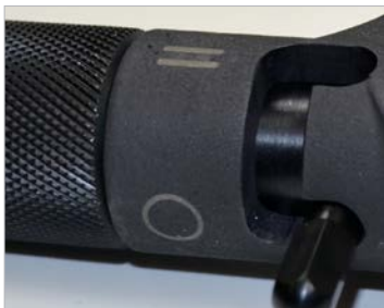
Convenient markings easily identify blade position settings to perform longitudinal and ring cuts.
