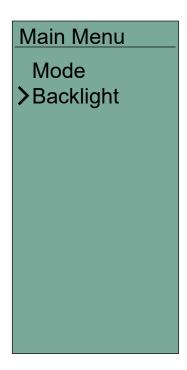
Use the Up/Down arrow buttons to move the cursor to the option you would like to explore. Press the Left arrow button to go back to the Main screen. Press the OK/Menu button or the Right arrow button to select an option.
