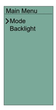
Use the Up/Down arrow buttons to move the cursor to the option you would like to explore. Press the Left arrow button to go back to the Main screen. Press the OK/Menu button or the Right arrow button to select an option.
