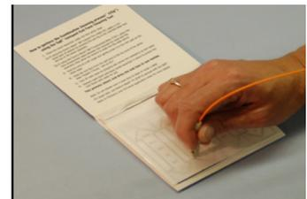
The wet/dry method (shown above) utilizes a lint-free pad and a fiber wash pen filled with a solution of alcohol. To use this method:
