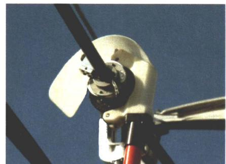
**Step #7.** Move the tool stop a distance away from the RMS tool equal to the required strip length. Turn the handle clockwise while applying pressure to the tool in the direction of the strip. The tool will strip more insulation and begin to self-feed after one turn.
