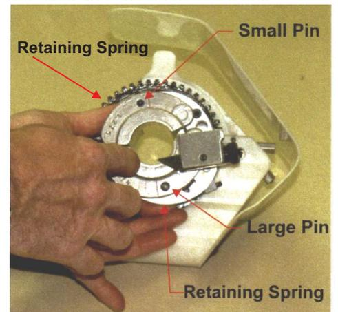
STEP # 4. Choose the bushing with the number that matches the cable gage indicating the cable size in the previous step. Insert the bushing into the tool head by pushing the retaining spring in and sliding the bushing into the bushing holder. The bushings will only go in one way because they have different diameter holes that fit on different size pins.
