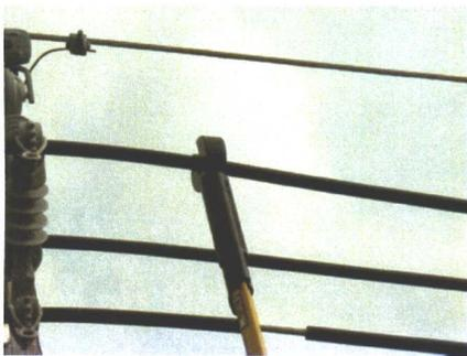
This gage shows correct bushing being used. Cable goes to middle of gage.
