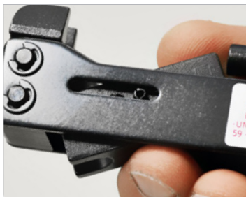
Unique pivoting block accommodates proper compression of connectors.
