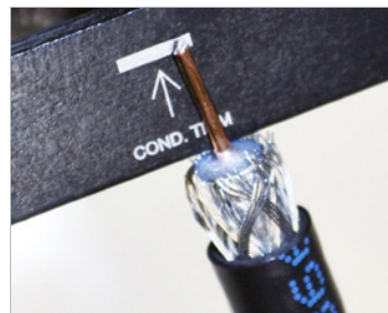
Center conductor gauge on tool body ensures proper preparation lengths.
