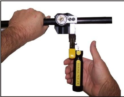
1. Grasp cable in one hand; depress lever on Banana Peeler and place the cutting blade at the desired scoring point. Spring-loaded jaws close, and blade penetrates the semi-con precisely to the set depth. Rotate tool around circumference of cable. Blade scores sheathing 360 degrees. Remove tool.
