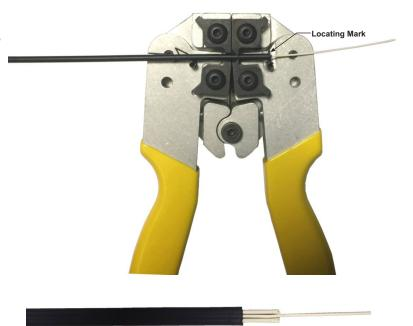
**4.** Squeeze the handles fully to cycle the tool and the specified length of jacket material will be removed exposing the GPR rods.
