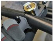
Ergonomic tool handle provides additional leverage during ring cutting operations.
