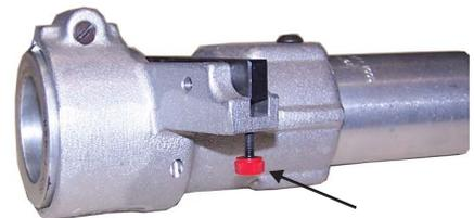
**Step 6.** A Blade Lock Screw is provided with all WS6 tools. After the blade is adjusted in Step 5, thread the lock screw into the casting. Turn until the end of the screw makes contact with the bottom of the blade to secure it from movement. Avoid over-tightening this lock screw.
