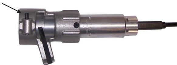
To remove the bushing, depress the lock release pin on the housing and slide the bushing out
