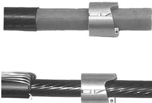
**Step 1.** Check the bushing by sliding it over the polyethylene insulation or over the semi-con on EPR insulated cable. The bushing should fit closely, yet still rotate easily on the cable.
