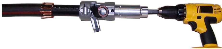
**Step 8.** The tool is ready for power operation as shown above, or can be operated manually.
