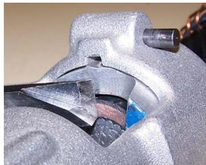
**Step 5.** Before stripping the insulation, adjust the blade edge to 1/32" (.79mm) - 1/16" (1.59mm) above the conductor surface by inserting the provided 1/16" hex wrench through the hole located beneath the tool blade. Turn the adjusting screw in the bushing to re-position the blade.
