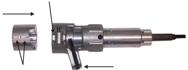
**Step 2.** To insert the bushing into the WS6, line up rib on the bushing with the slot on the WS6 housing. Raise the cutting blade by depressing outer end and insert the bushing until it locks into place.
