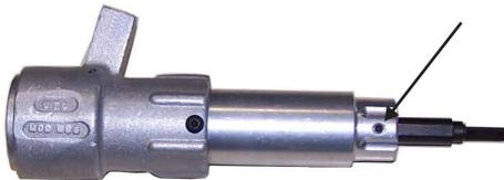
**Step 3.** To adjust the stop bar for desired length of conductor exposure, loosen the set screw located at the back end of the tool with a 1/8" hex wrench. Adjust the stop bar to the desired length of insulation to be stripped and tighten the set screw. Up to 5-1/2" of insulation can be removed with this tool.
