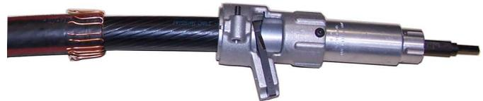
**Step 4.** Insert the cable into the WS6 until it comes in contact with cutting edge of the blade.
