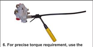
6. For precise torque requirement, use the TW series torque wrench. Back end of S-200 is slotted to engage the wrench.
