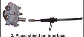
Place shield on interface.Place tool on cable as shown.
