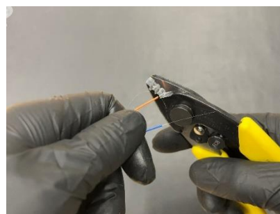
5. Use the smallest notch on the CFS-3 for individual fiber, or largest notch for flexible buffer tube.
