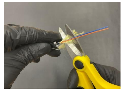
6. The KS-2 shears are good for any Kevlar strength fibers.
