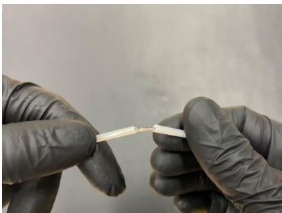
4. Snap the buffer tube to expose the inner fibers. Clean if necessary.
