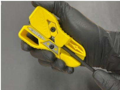
1. Remove the toner wire with the MB03-7120.
