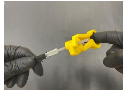
3. After trimming away the jacket and buffer tubes, ring twice with the FTS scoring tool.
