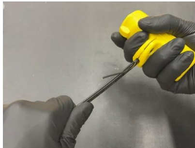
2. Use the MB04 Twister drop splitter to score each side and peel away the jacket.
