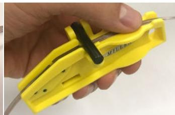
Close the clamp. Apply even thumb pressure on the ribbon, in front of the blade. This ensures an equal tension on all the fibers.
