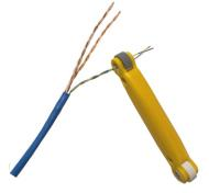
2. Continue turning the guide roller and allow the tool to self feed and unwind the twisted pair.
