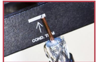
Center conductor gauge on tool body designed to ensure proper preparation lengths.
