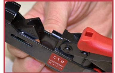
Unique pivoting block accommodates proper compression of various connector types.
